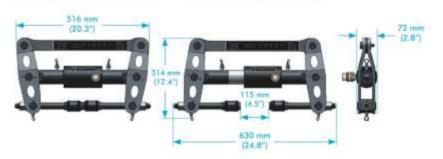
Tool Weight: 21.5 kg (47.3 lb) Case Weight: 9 kg (19.8 lb) Gross Kit Weight: 40.5 kg (89.3 lb)
