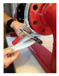
Then feed the free end back through the buckle, in between the two rollers.
