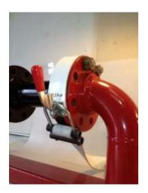
The flange spray deflector belt can be used for the following:
