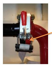
Arrange the buckle so that the flange access gap (pictured left) is pointed in a safe direction. The flange access gap allows the operator to use a pry bar to break the seal between flanges.
