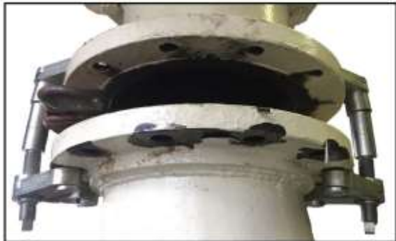
SMP Valve-Out Tool Works Great in the Vertical Position Too
